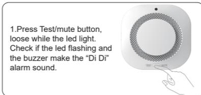
1. Press Test/mute button, loose while the led light. Check if the led flashing and the buzzer make the "Di Di" alarm sound.
