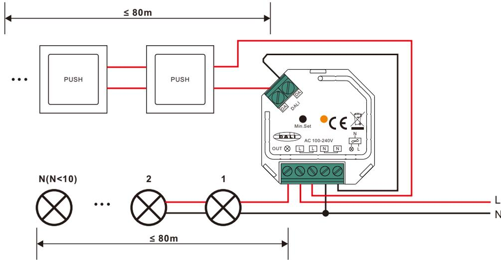
This phase dimmer adopts trailing edge dimming (reverse phase control), please make sure the connected loads support reverse phase control. Please refer to the user manual of the load or consult the supplier of the load.
