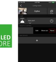
From your ZigBee controller or hub interface, choose to delete or reset the remote as instructed, indicator flashes 3 times quickly to indicate successful removing.
