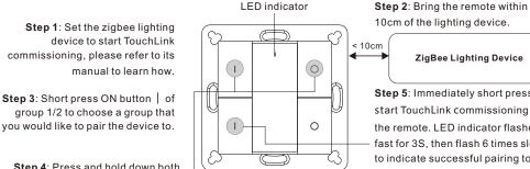
Step 4: Press and hold down both buttons until LED indicator turns on.
