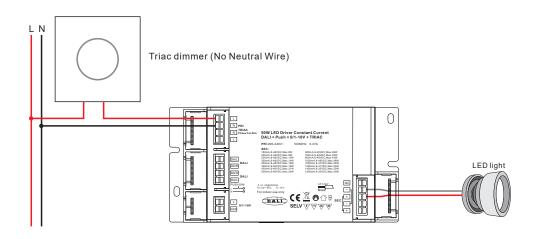
1.2 One Triac Dimmer to Control Multiple Drivers Simultaneously
