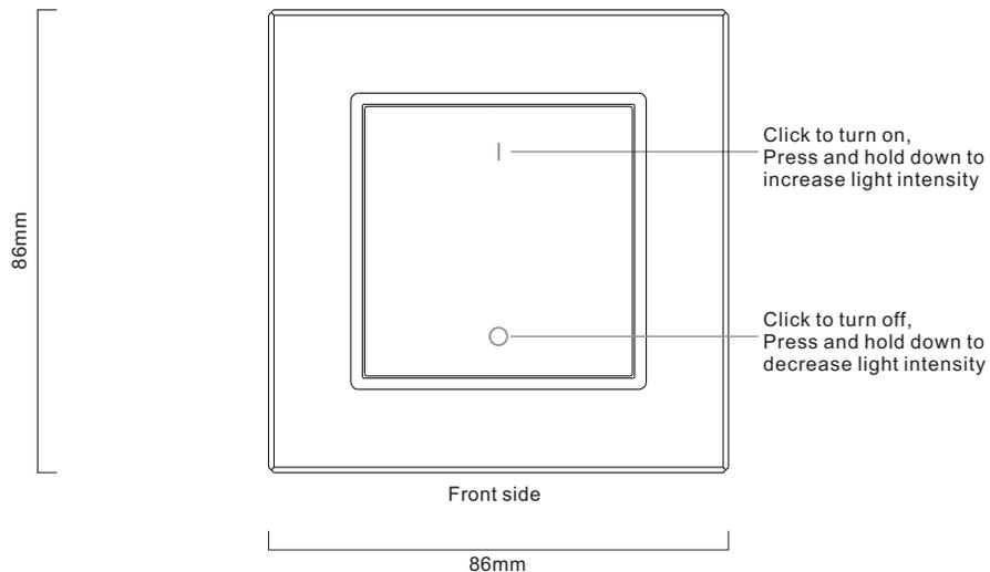
The remote control can be fixed on the wall with 3M glue or screw.
